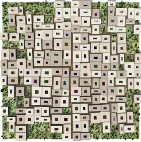
Fig. 19. Final plan view rendering of the fractal kasbah showing final shapes in the form of buildings and garden spaces. The amount of garden spaces increases towards the edges of the system.
