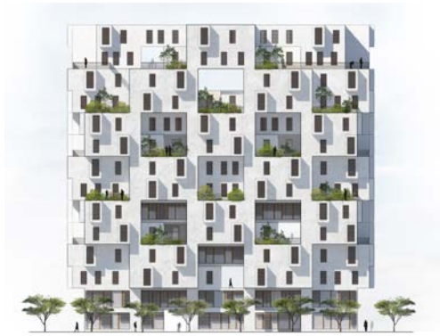
Fig. 6. Front elevation. Parts of the facade protrude, while others are set back, in order to provide a high ratio of shaded facade parts. In setbacks at the bottom of the structure, windows are large in order to provide daylight in interior spaces. Higher up, windows in setbacks are smaller to minimize direct sunlight in interior spaces. Not to scale.
