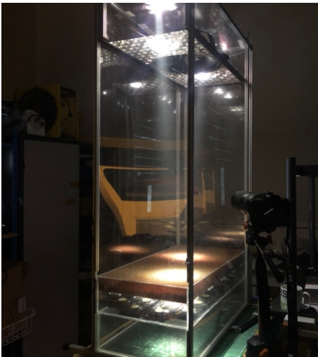
Fig. 4 – A prototype at scale 1/3 of installation, currently used for first experiments at the LadHyx, Polytechnique Paris-Saclay, France. The walls of this version are made of rigid polycarbonate panels. The small fans that produce the airflows can be seen on the bottom, just under the honeycomb panel that parallelize the streams. On the top appear the infra-low frequency loudspeaker that is used to study the effect of sound waves on the mist configurations.
