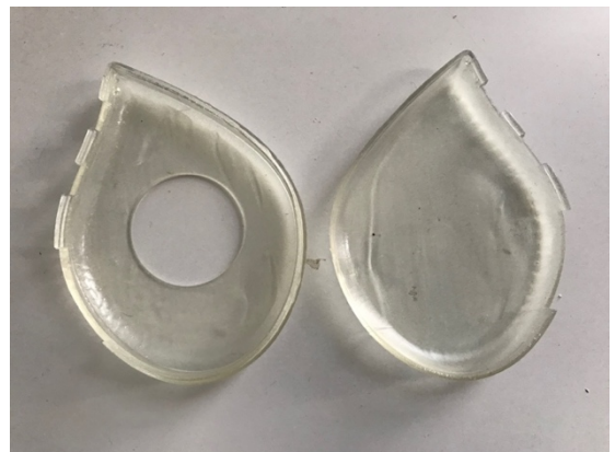
Figure 4: Clear resin 3D print of Sound Drop casing.
