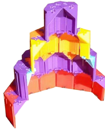
Figure 3: example of a four-layer muqarnas built with 3D printed units.
