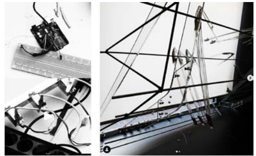
Figure 5 Exo components' site-specific assembly. a. Arduino microcontroller and electronic integration and the architectural montage of servo motors. b. bearing construction and kinetic components ("feathers"); Kolektiv Gallery , Author: Dragana Ćirić; Software integration, electronic and technical support: Aleksandar Popović (Karkatag Kolektiv); Photography: Nikola Abramović
