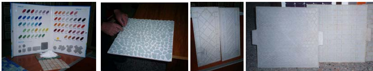
Figure 12. Glass tesserae and template trays used to produce mosaic tiles and panels.
