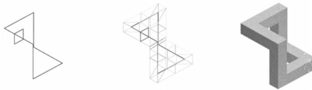
Fig. 7: the toroidal EI-form as extrusion
