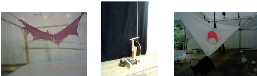
Fig. 5-6-7 First experimentations on tensed membranes. In the middle: one of the motors.
