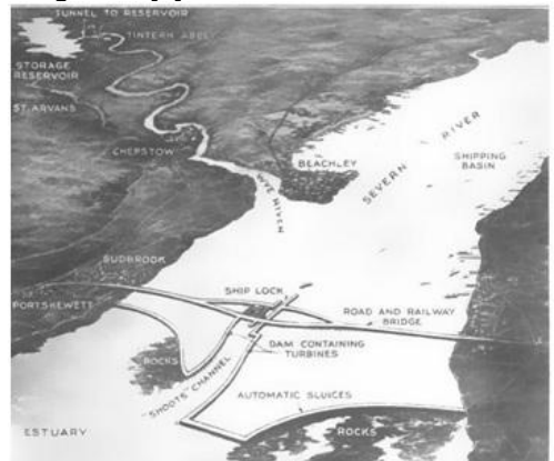
Fig. 6 Woodruff (1921) A diagrammatic aerial view of the Severn River tidal-power project: In the foreground is the 2.5 mile dam with its automatic sluice gates; behind it the shipping basin of 27 miles; in the upper left corner, the big storage reservoir of the secondary plant, 10 miles away on River Wye. In Popular Mechanics, March 1921
