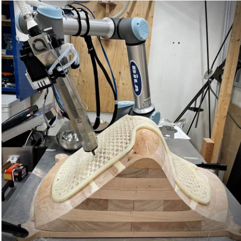
Figure 1: Robotic 3D printing setup.
