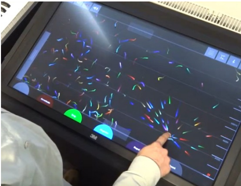
Figure 1: The TouchNoise system sonifies a particle system. Particle motion is influenced by multitouch interaction.
