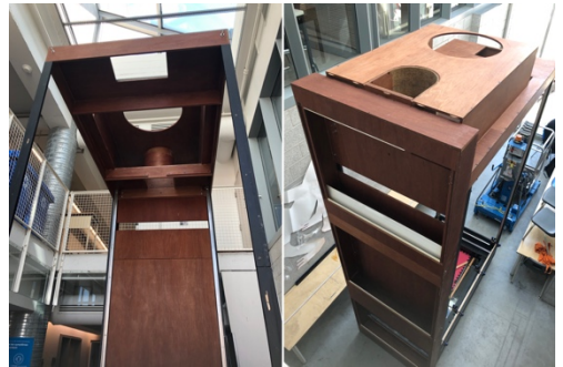
Fig. 5 – The full-size version of the installation, currently being built at the UQAM School of Design in Montreal. The double wall on the back houses the mist recirculation system. The openings on the top will house a subwoofer and a planar laser. Three of the four walls will be made from mirror films; the front one will be transparent.
