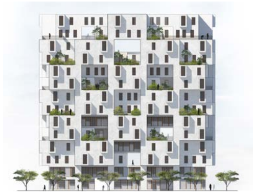
Fig. 6. Front elevation. Parts of the facade protrude, while others are set back, in order to provide a high ratio of shaded facade parts. In setbacks at the bottom of the structure, windows are large in order to provide daylight in interior spaces. Higher up, windows in setbacks are smaller to minimize direct sunlight in interior spaces. Not to scale.
