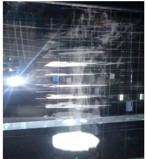
Fig. 7 – Mist structure materialized by planar lights.
