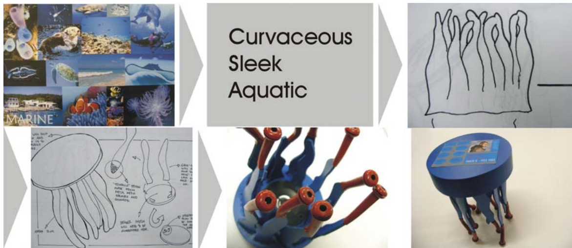
Figure 6 Illustration of the procedure of designing a CD player for Marine Biologists following Method 2
