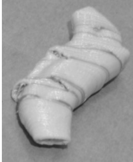
Photo. 7: Zebra crossing as result of some “Part” fibers is accidentally replaced by “Supports” fibers
