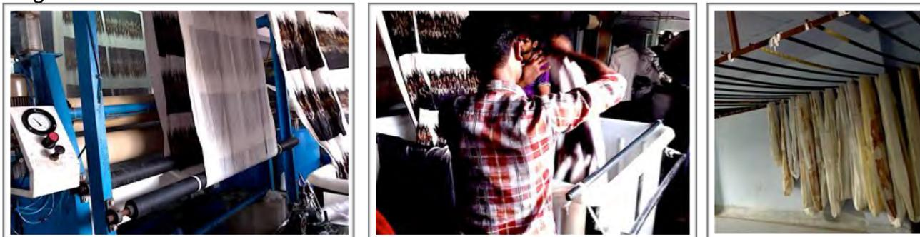
Benefit of aqueous-based sublimation ink is that there are no hazardous components as it is found in UV-curable, solvent and in latex inks. Direct fabric printing using disperse ink on uncoated fabrics offers maximum advantages. These prints can be seen from both sides of the fabric which is an essential quality of digital printing. These prints get more profit, with an 'eco-friendly' label and with a higher quality. Other fabric and ink combinations cannot allow this.
