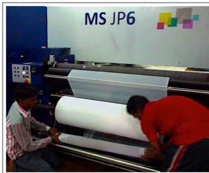
Most used fabrics for digital printing is a polyester based fabrics. The printing process should match with type of ink e.g. low energy sublimation (dye-sub), high energy sublimation (also known as disperse direct), reactive, acid and pigment. The ink chemistry should fit the requirements of the fabric (nylon, polyester, silk, cotton). On the bases of choosing fabric and ink combination, the process followed for heat-press sublimation, infra-red fixation or steaming.
