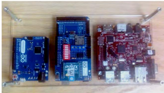
*Figure 5 – XEPA “Brain” without front acrylic cover and processor interconnects*
