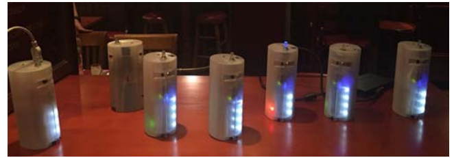
Fig. 3 – The Harmonic Lanterns at Mende. These devices are individually held and connected to a headset. Their role was to geolocalize the visitors and to play the musical timbre corresponding to their position, with a 10-cm precision. Their design and morphology were almost only determined by functional and practical considerations.
