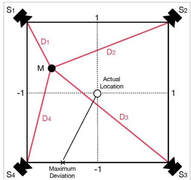
Figure 6. Four virtual sound sources ( $S_1$ – $S_4$ ) are placed in the corners of a square whose size is based on the maximum deviation. The waypoint position data control the position of the virtual microphone ( $M$ ). The resulting distances ( $D_1$ – $D_4$ ) form the parameters for the sound processing.
