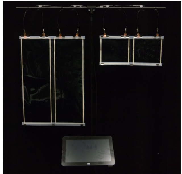
Figure 1: Appearance of the Installation. Shown in this photograph are two piezoelectric films of different size that are suspended from a horizontal bar. Attached underneath the films is a touch screen that runs a simple graphical interface and that allows visitors to alter some aspects of the digital signal processing that forms part of the acoustic feedback.
