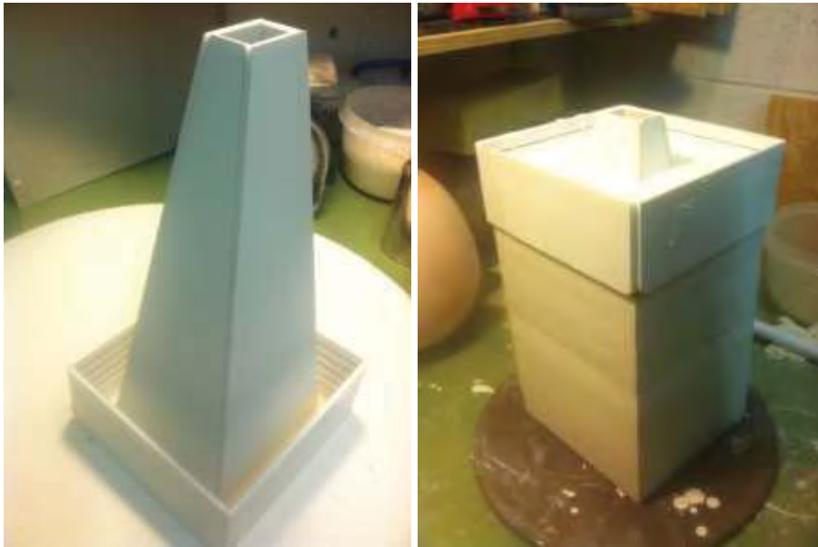
(1.1) Foam core original form with repositionable containment box in lowest position, without plaster layers.
