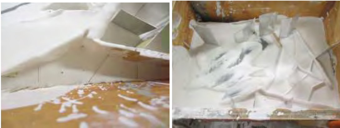
(6.9) Example of metal shim (not shown) pushed into gelling plaster and then pulling it back out when plaster has hardened enough not to close back up (seen here as the thin dark lines). These divisions will not be part of later layers.
