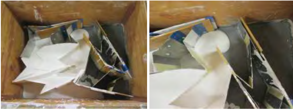
(6.7) Plaster pouring targets different areas of mesh, which fills them earlier. This means subdivisions will be at various levels.
