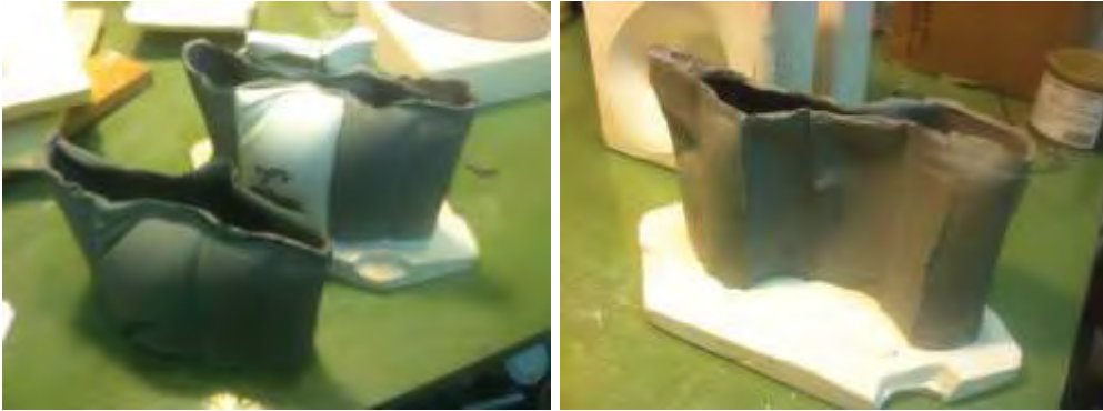
(5.12) Comparison of two castings created from same mold, full form (foreground) and partial form.
