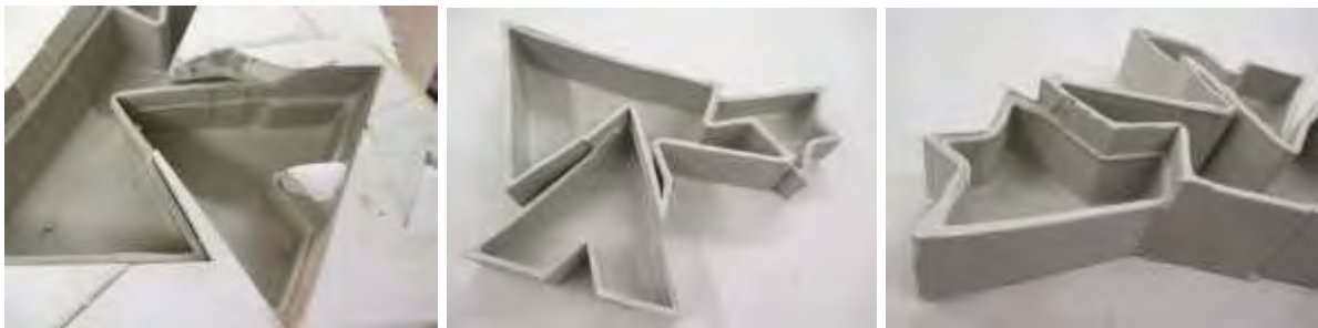
(3.7) Next set of open areas created for second casting filled to shorter level. Note thicker wall on newly exposed (most absorbent) plaster surfaces, and thinner wall fused to original wall (less absorbent).
