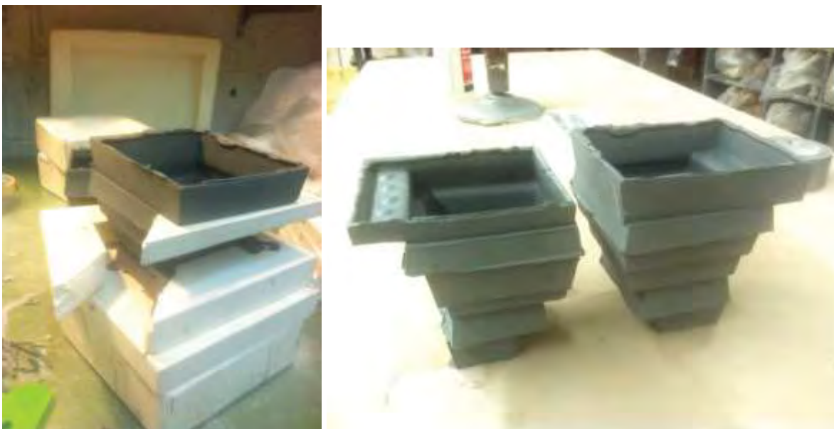
(1.7) Unmolding in progress for casting with "flip," "skip," and "slide" variations. Note split in each layer that solves draft angle problems. (1.8) Unmolded castings when twelve layers of original mold are divided into two groups ("skip") and reoriented ("flip" and "slide").
