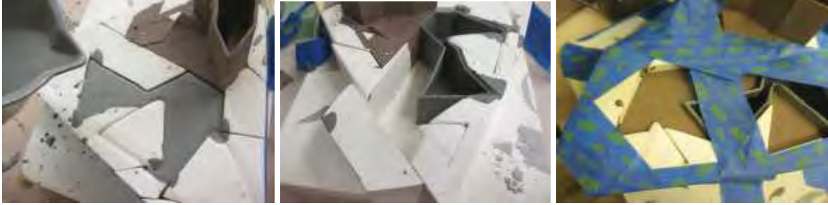
(3.13) Second pour of white slip (seen as grey shiny liquid in photo) in newly exposed containment.
