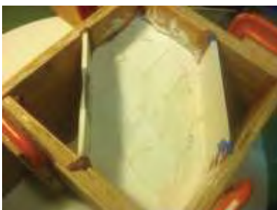
(5.6) Nine cells fully filled with plaster containment pieces around them, scraped
