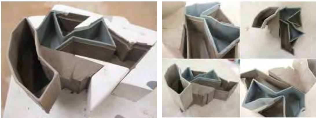
(3.16) Entire casting shown partially unmolded.
