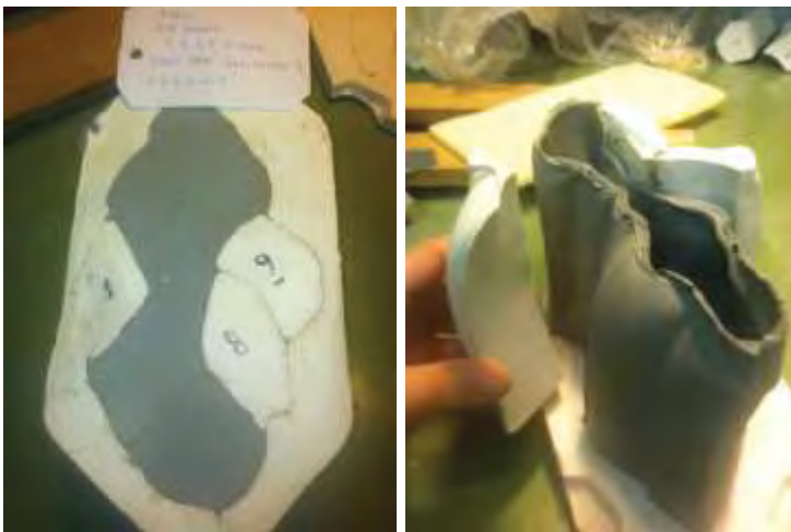
(5.10) Form that results when plaster pieces 1,8,9 remain in mold, creating union of pieces 2,3,4,5,6,7 (shown from bottom of mold)
