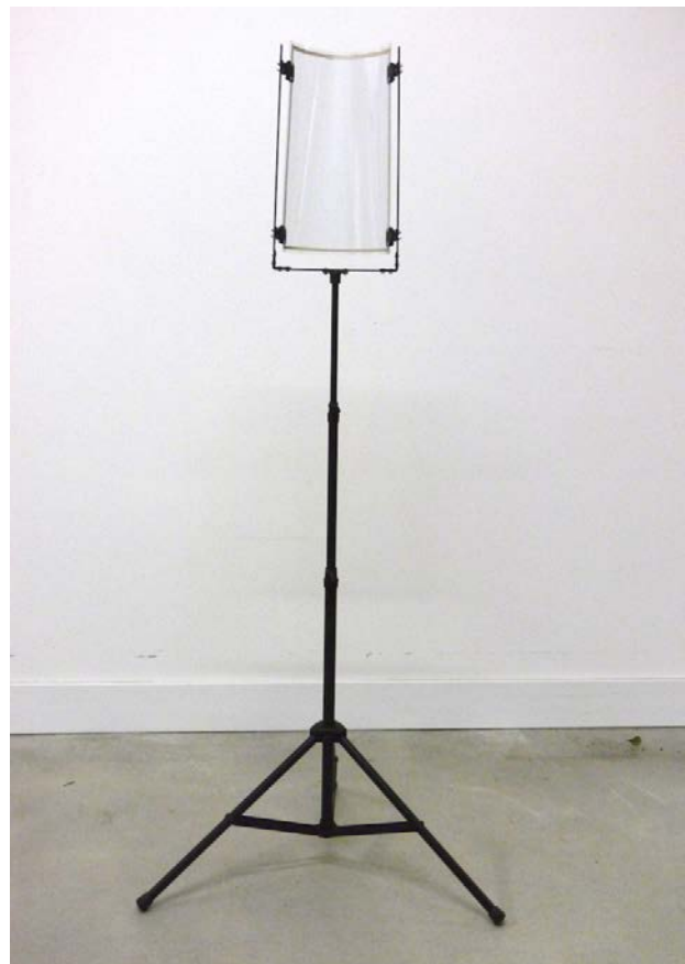
Figure 1. Piezoelectric speaker films mounted on the foot part of a music stand form the sounding objects of the installation.
