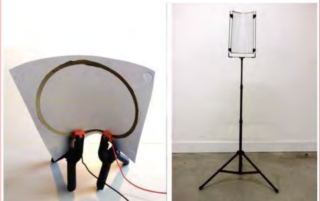
An early prototype of a piezoelectric speaker film (left) and one of the actual objects of the installation (right).
