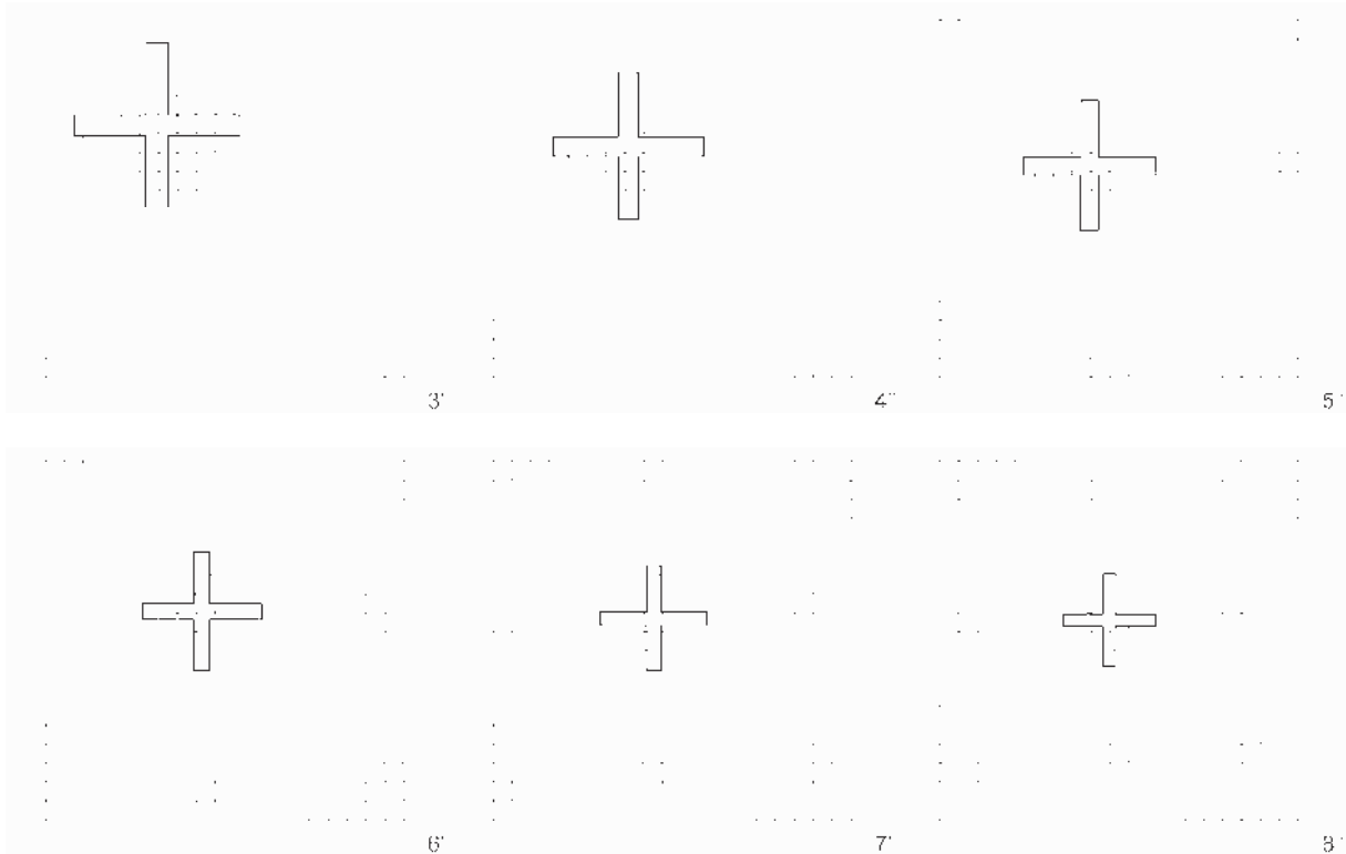
Fig. 9. Image blur and magnification showed by a special case of moiré type (1,0,-1,0). The sample dot is the shape “+”. Illustration by author.
